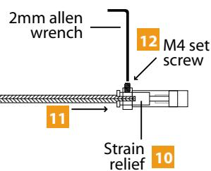
**10** The strain relief slots should be rotated 90° away from the M4 set screw.
